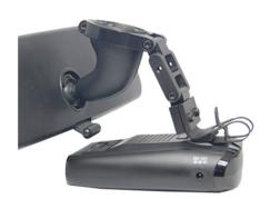
STEP 4 - Install the radar detector and slide the mount upwards leaving approximately 1/8" of clearance between the mount and the windshield. Rotate the mount untill the radar detector is level from side to side and tighten the top screw.
