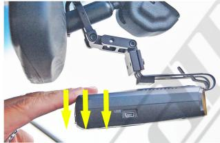
push the RD downward just enough for your finger to fit between the RD and mirror. Do not push down more than what is needed.
